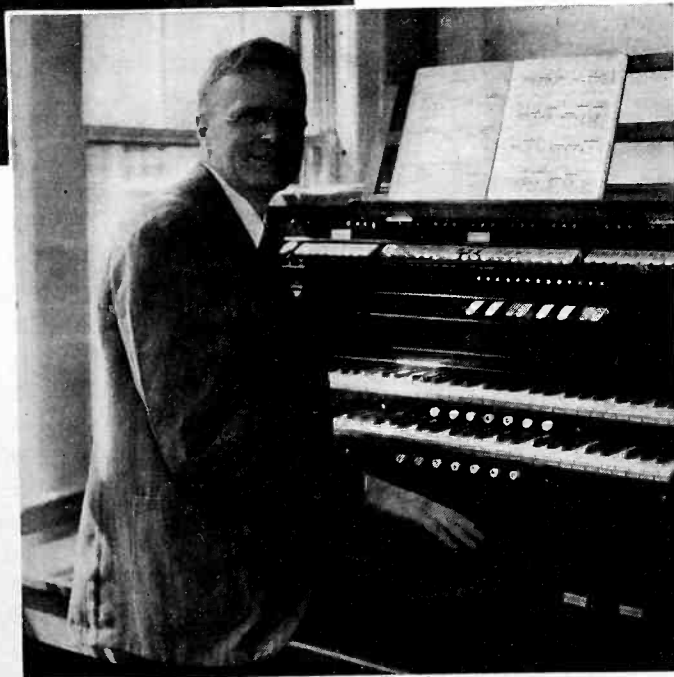
Captain Richard H. Ranger at the keyboard of his Ranger-tone electric organ. Fixed-ratio alternators provide the source of the fundamentals and harmonics, which can be combined in various proportions, creating a wide range of effects, including some strikingly new musical characteristics
