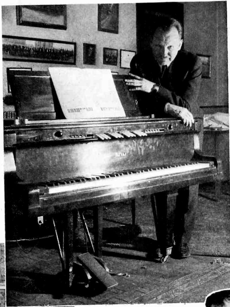
Benjamin F. Miessner and his electronic organ-piano. The piano-strings when struck, produce vibrations, which are amplified, modulated and recombined, and heard through a loudspeaker, producing many new and unusual effects
